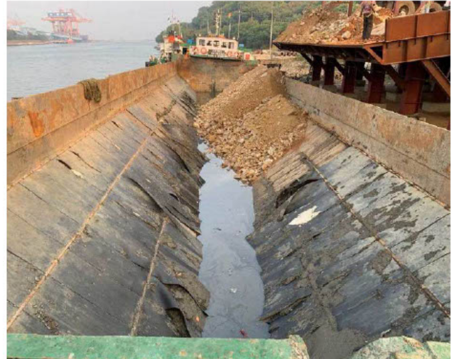
Supply Of Reclamation material Through Split Barge to VCT-2 Project Site. (VCT-2)
